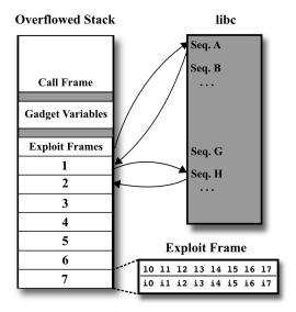
Fig. 31. Function Call Gadget Stack Layout
