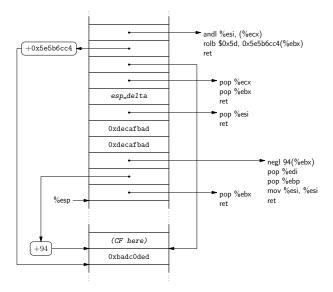
Fig. 17. Conditional jumps, task three, part one: Convert the word (labeled "CF here") containing either 1 or 0 to contain either <code>esp\_delta</code> or 0. The data word labeled <code>OxbadcOded</code> is used for scratch.
