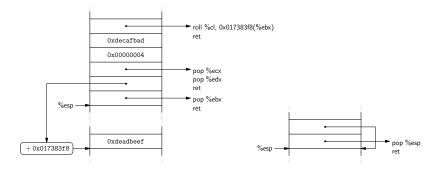
Fig. 13. Rotate 4 bits leftward of memory word.
